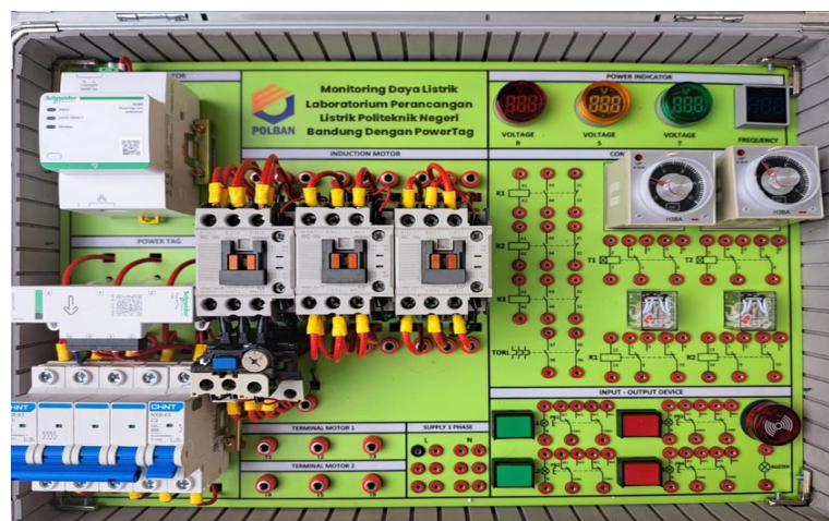
Figure 4. Electric Power Monitoring Simulator
